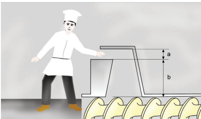
Picture 10: Workers' access to the hazardous area must be prevented by protective devices. The entrance height "a" to the machine is intentionally designed in such a way that human hand cannot be pulled in. In case when the height "a" allows the entrance of the hand, then "b" must be that long to prevent the hand reaching the knife.
