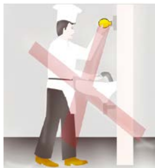
Picture 8: Simultaneous contact of the body under voltage and eg. a metal waterpipe generates the risk of electric shock. When replacing the bulb or opening electrical devices, first thing to do is to switch off the voltage. Electric consumers and appliances must be regularly maintained, periodically reviewed and examined by a qualified person.
