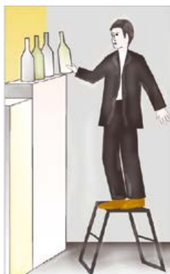
Picture 20: Stepladders are correct only if whole, if the bars are built-in, legs secured to each other by a rope, chain and similar. All ladders must be manufactured according to the Safety at Work regulations, with standard and certificate mark. Only one person at a time should stand on a ladder. Hands need to be free. Tools should be carried in a waist bag. When climbing, bars should be held by hands. If there is no handrail (as on picture) the stepladder is supposed to have two stairs at most.
