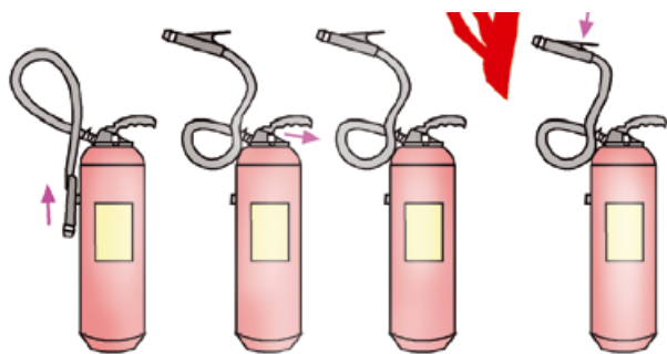
Picture 33: Activating the procedure of the extinguisher for initial fire protection: 1. bring the device to an acceptable distance from the fire, hold the nozzle, 2. pull the safety fuse out, 3. direct the nozzle to the fire, 4. press the lever on the device and the lever on the hose nozzle (if having any)
