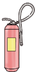
Picture 32: Extinguisher under constant pressure for initial firefighting uses powder. Its parts are the tank, the activation lever, the safety fuse, the hose with nozzle and often a manometer, too. The extinguisher must be labeled with the expiry date information. It should be checked at least once per year by an authorized legal entity. The tank's constant pressure is about 15 bar.
