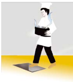
Picture 18: Fall into a floor opening while carrying a view-hiding load. All floor openings must be enclosed with fences and marked. Paths and passes, stairs and other movement areas need to be clean, without obstacles or bulges, and well-lit.
