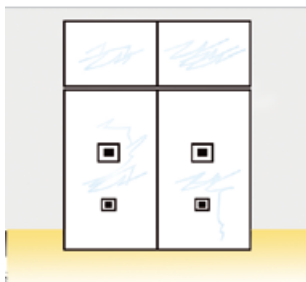
Picture 19: Stickers should be placed on the glass door in order to make it visible. The door must be opened outwards in the exit direction due to evacuation. It should not be locked.
