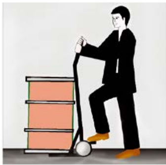
Picture 13: Trolley parts must be designed in such a way that neither the trolley nor the load can hurt the user. The trolley should be loaded uniformly in order to not disturb stability. When loading, push firmly the foot on the axle of the trolley to the ground to prevent it from moving. Check the trolley's permitted load carrying capacity.
