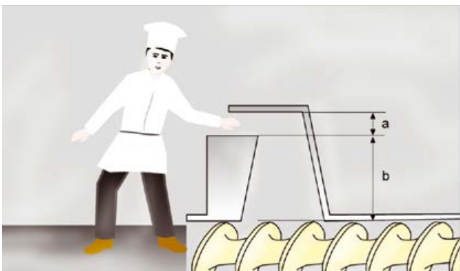
Picture 10: Workers' access to the hazardous area must be prevented by protective devices. The entrance height "a" to the machine is intentionally designed in such a way that human hand cannot be pulled in. In case when the height "a" allows the entrance of the hand, then "b" must be that long to prevent the hand reaching the knife.
